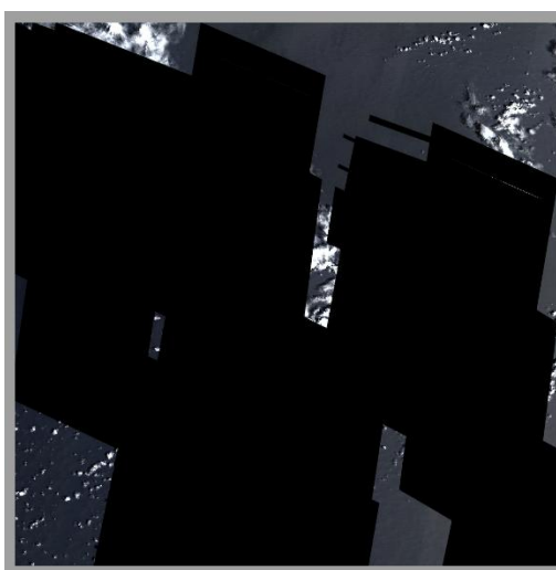
Figure 2-14 – L2A TCI image of a tile processed with a Quality Mask masking the defective pixels of different affected bands.
